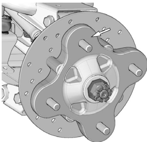
3. If applicable, remove CV joint protectors.
