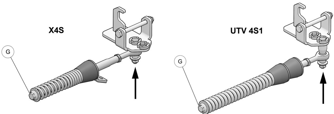
9. Inspect the rear Track Systems and ensure that all mounting bolts were correctly tightened during installation. Lower the vehicle on the ground and proceed to install the front Track Systems.
