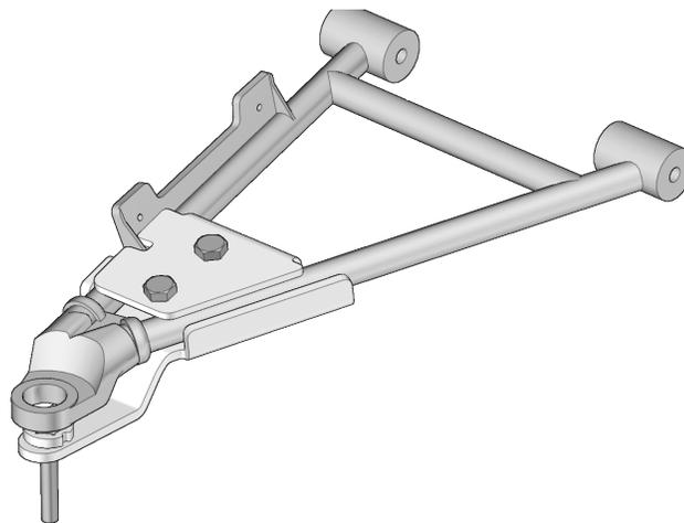
6. Using the wheel nuts (12) provided, secure undercarriages to front wheel hubs. The procedure and precautions are the same as for rear units. See Figure 8 for reference.
