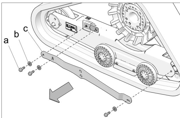
1.1 Remove bolts (a), washers (b) securing rigid suspension anti-rotation brackets (c) on System's rear undercarriages.
