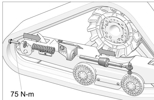
2.5 Install new stabilizing arms on frames as shown above. Assemble the different parts of the new arms in the order and direction indicated.
